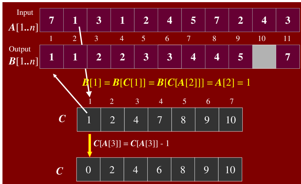
Figure 5.18: A[2] placed in output array B
