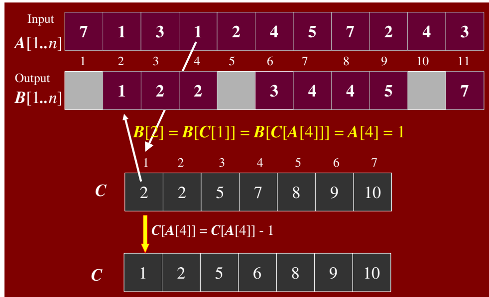
Figure 5.16: A[4] placed in output array B
