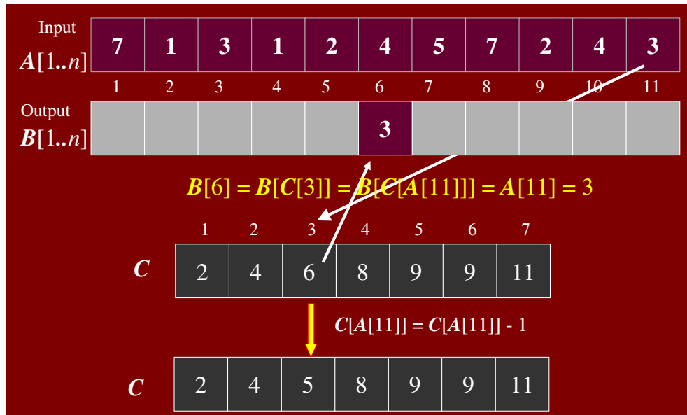
Figure 5.9: A[11] placed in output array B
